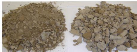
**Fig 1: Recycled Aggregate Before and after Sieving**
