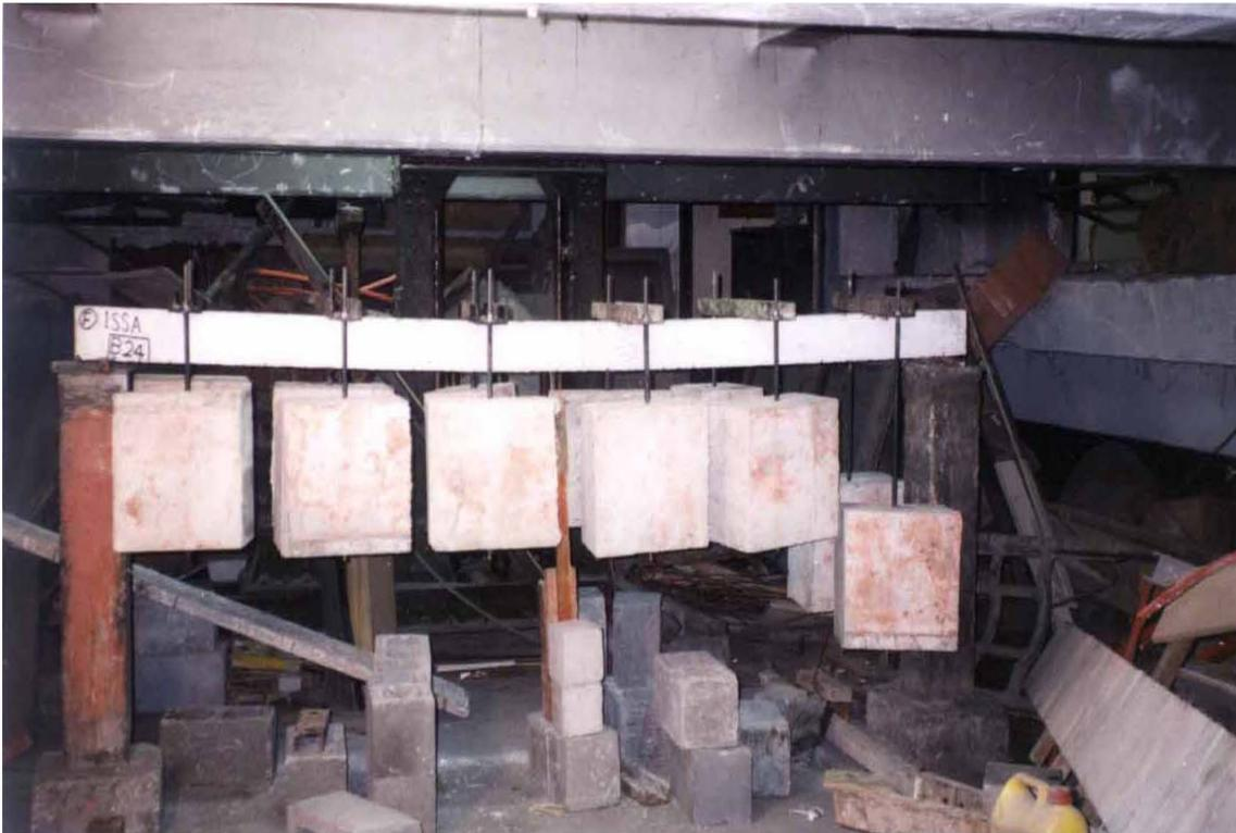
Figure (1): Sustained loading of Beam B5
