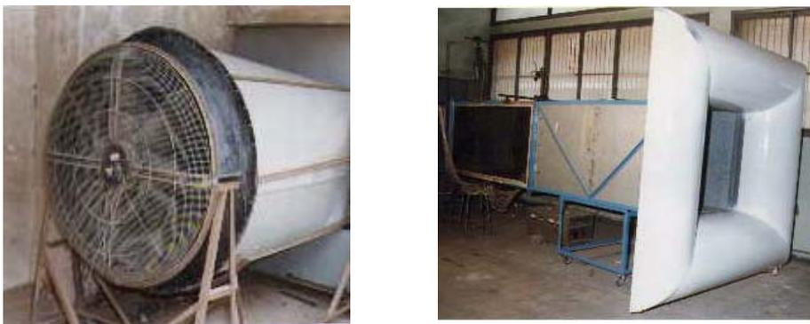
Fig 1-b A photograph of the Wind Tunnel and driven Section
