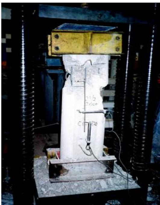
Photo (5) Mode of failure of column
