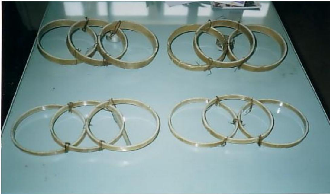
**Photo.1 : Configuration of the Interlocking "GFRP" Slices Used as Lateral Confinement for Group (B)**
