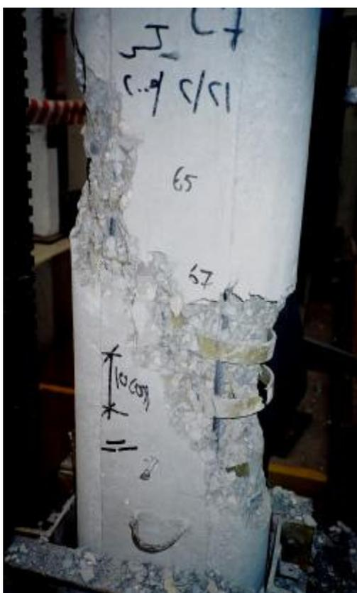
Photo (7) Mode of failure of column
