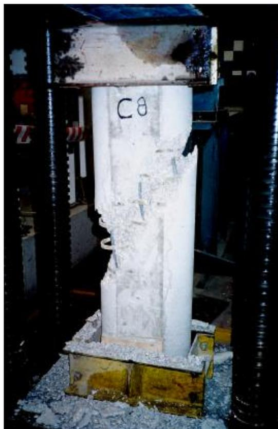
Photo (8) Mode of failure of column
