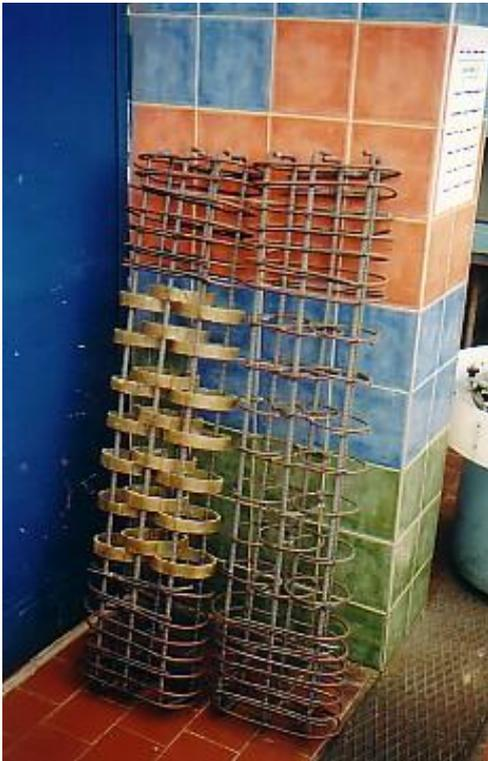
**Photo 2. Reinforcement Configuration of Columns C7-GF10 and C3-CS10**
