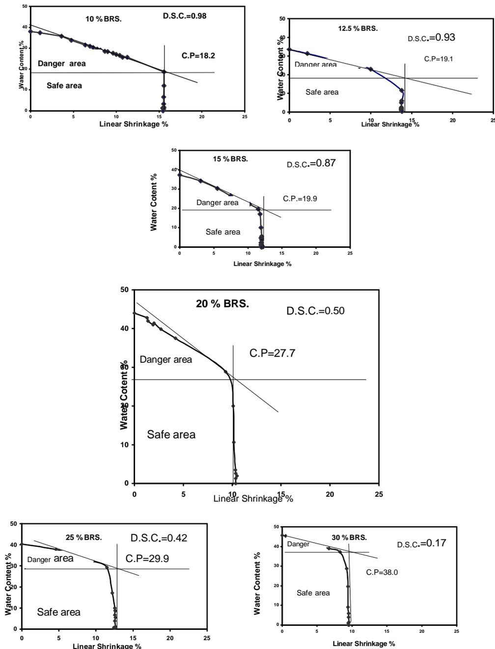
**Fig. 5: Bigot's Curves of the Studied Clay Specimens with Different Percentages of Burnt Rice Straw (BRS) Additives.**
