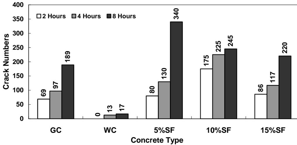
Fig. 1: Number of Cracks with Time for Concrete with Silica Fume.
