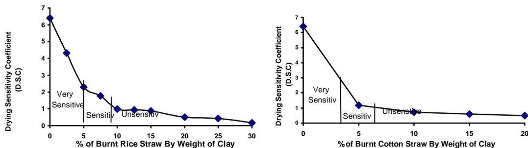
**Fig. 7: Relationship between the Percentages of Burnt Rice and Cotton Straw (BRS) and (BCS) within the Studied Clay Specimens and the Drying Sensitivity Coefficient (D.S.C).**
