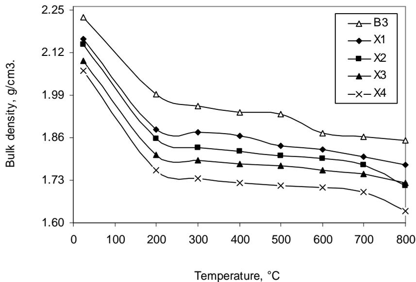
**Fig. 7: Bulk Density of OPC and Composite -Filled Cement Pastes as a Function of Firing Temperature up to 800°C**
