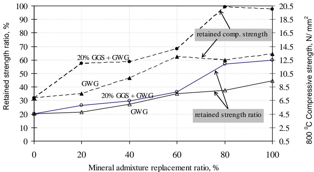
**Fig.6: Retained strength after 800 °C heat exposure**
