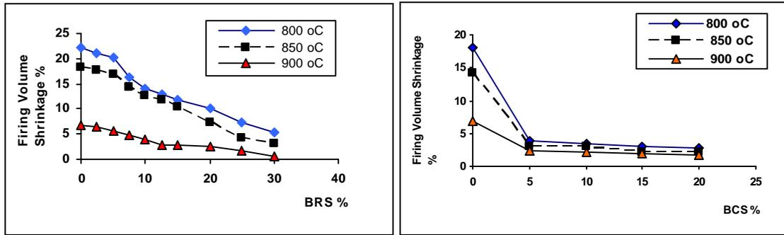
**Fig. 9: Firing Volume Shrinkage of Clay Specimens Fired at 800, 850 and 900 °C with Different Percentages of Burnt Rice Straw (BRS) or Burnt Cotton Straw (BCS).**
