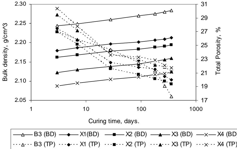
**Fig. 3: Bulk Density and Total Porosity of Composite - Filled Cement Pastes as a Function of Curing Time Up to 360 Days**
