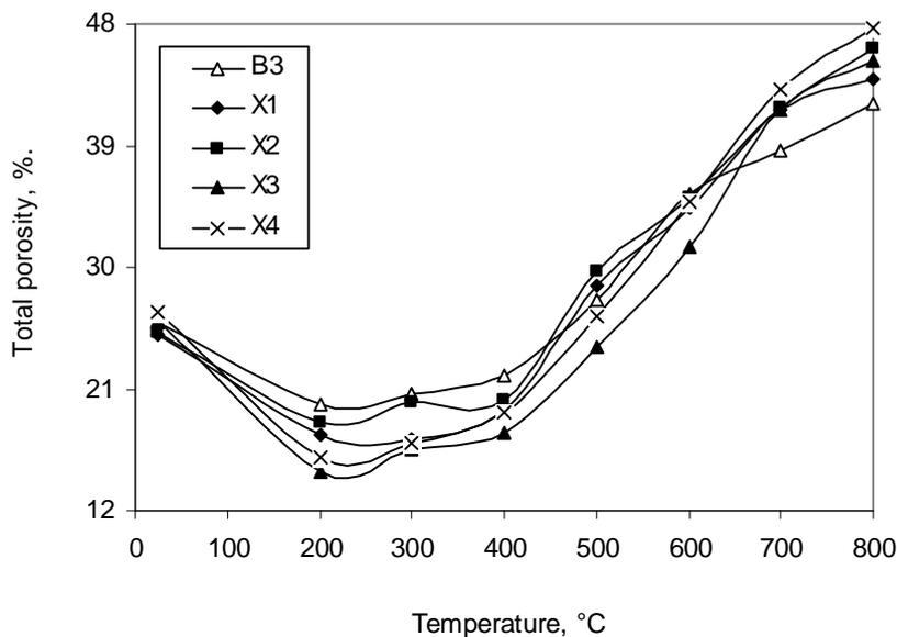
**Fig. 6: Total Porosity of OPC and Composite -Filled Cement Pastes as a Function of Firing Temperature Up to 800°C**
