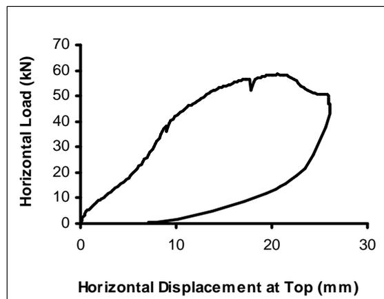
**Fig. 9: Horizontal Load versus Horizontal Displacement for Wall WG**
