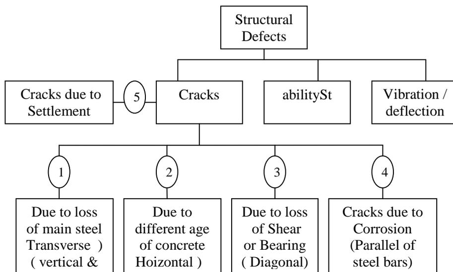
Fig. 3: The Type of Structural Defects According to its Causes.
