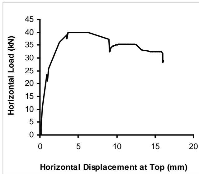
**Fig. 3: Horizontal Load versus Horizontal Displacement for Wall WP**
