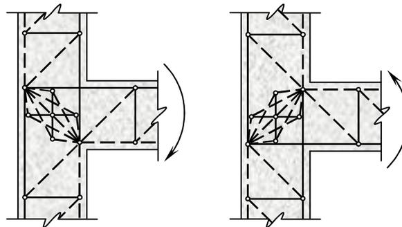
Fig. 2: SST Model by Hwang and Lee [12]
