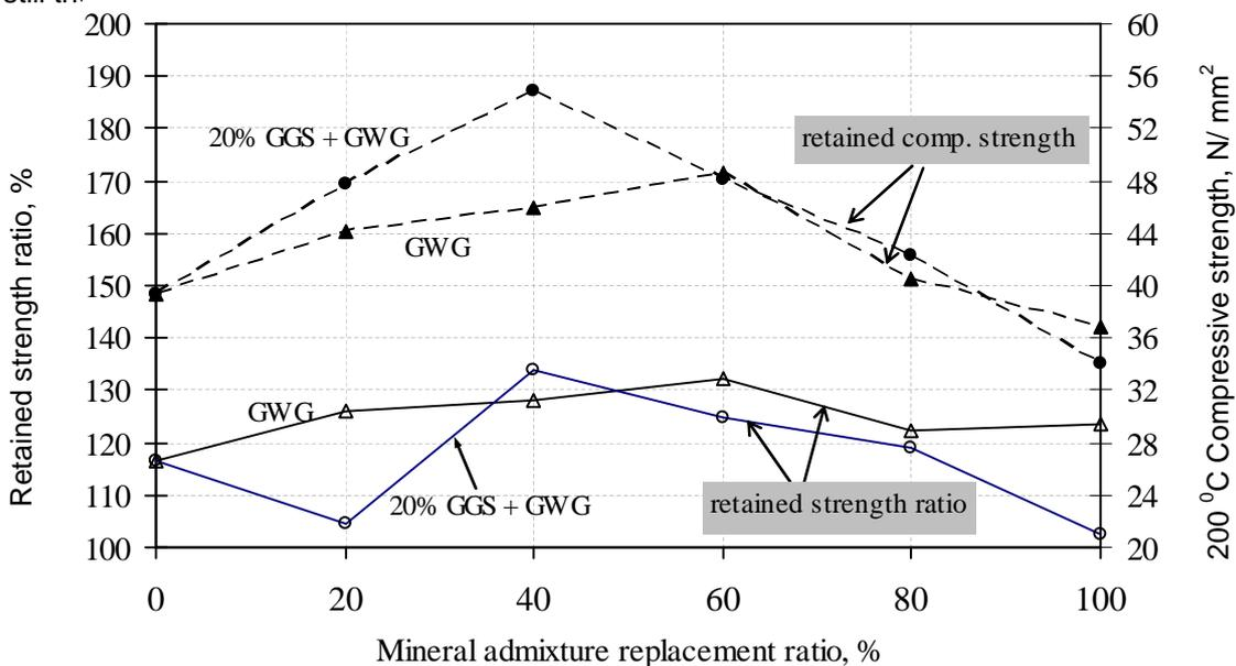
**Fig.4: Retained strength after 200 °C heat exposure**
