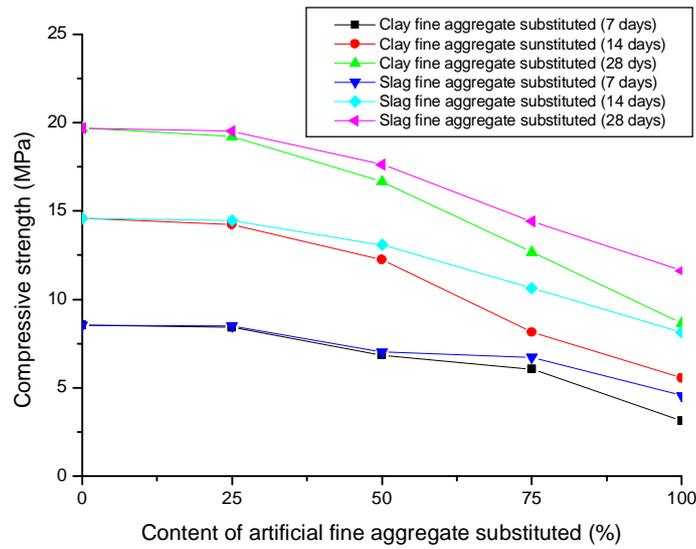
**Fig. 3: Variatin of Compressive Strength of Mortars as a Function of the Quantity of Artificial Fine Aggregate Substituted**
