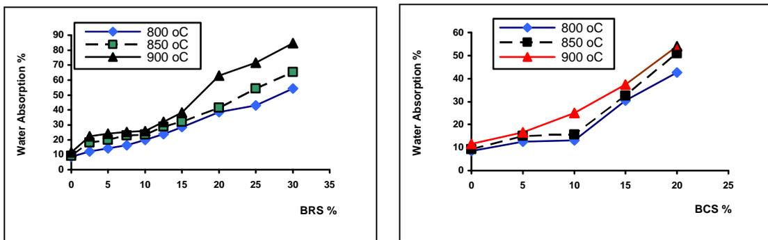
Fig. 12: Percentages of Water Absorption of Clay Specimens Fired at 800, 850 and 900 °C with Different Percentages of Burnt Cotton Straw (BCS) Additives.
