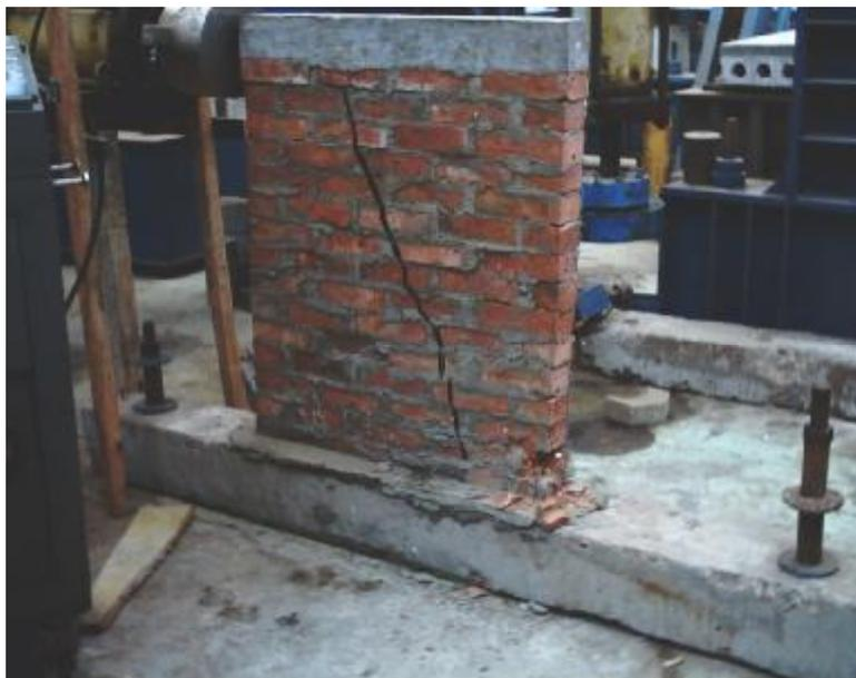
Fig. 12: Crack Pattern of Wall WG
