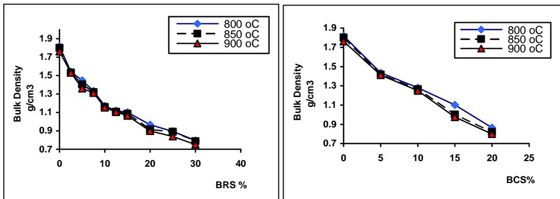
**Fig. 10: Bulk Density of Clay Specimens Fired at 800, 850 and 900 °C with Different Percentages of Burnt Rice or Cotton Straws (BRS) or (BCS).**
