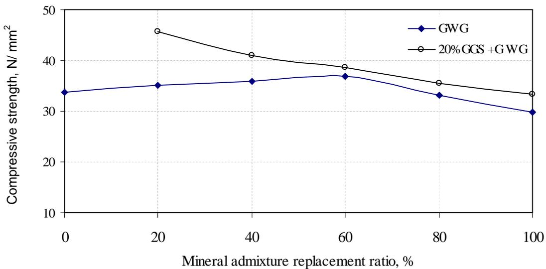
Fig. 2: 28 Day Compressive Strength of the Investigated Mortar Mixtures
