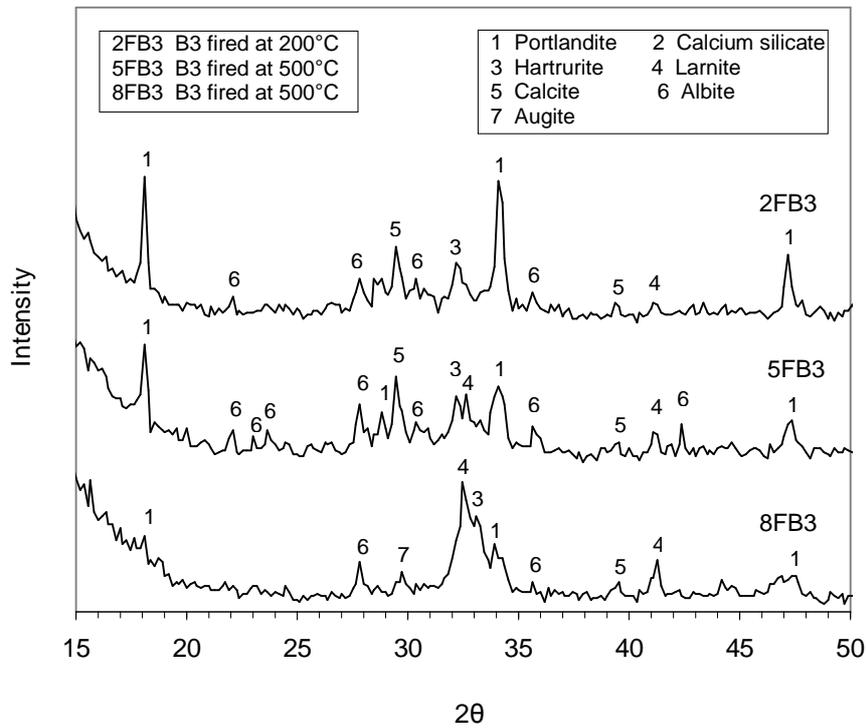
**Fig. 9: XRD Patterns of Pozzolanic Hardened Cement Pastes Made from OPC and 20% Basalt Fired at Different Temperatures Up to 800°C**
