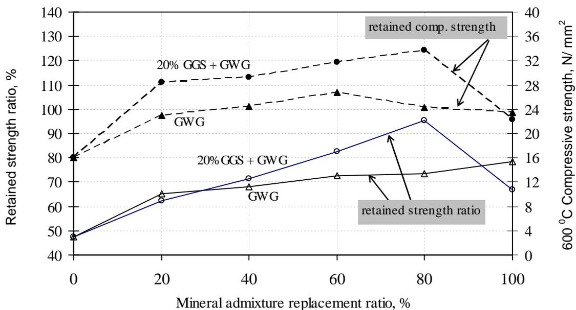
**Fig.5: Retained strength after 600 °C heat exposure**
