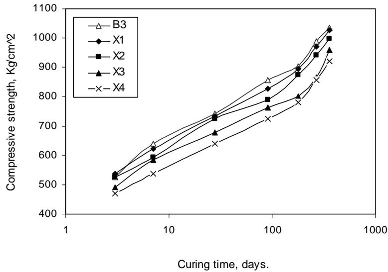
**Fig. 4: Compressive Strength of Composite - Filled Cement Pastes as a Function of Curing Time Up to 360 Days**
