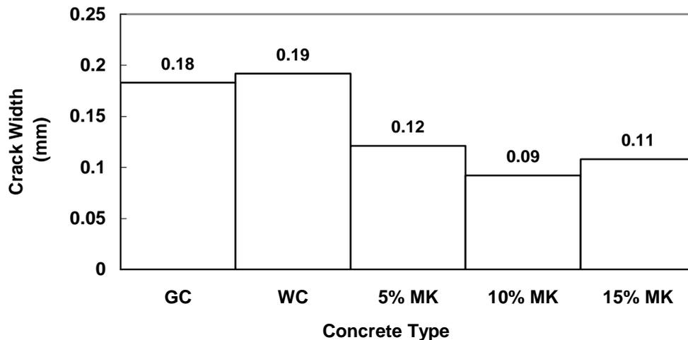
Fig. 4: Average Crack Width at 8 Hours for Concrete with Metakaolin
