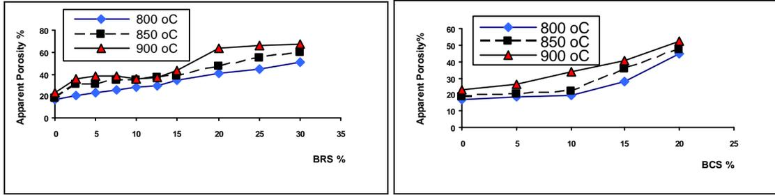
Fig. 11: Apparent Porosity of Clay Specimens Fired at 800, 850 and 900 °C with Different Percentages of Burnt Rice and Cotton Straws (BRS) or (BCS) Additives.
