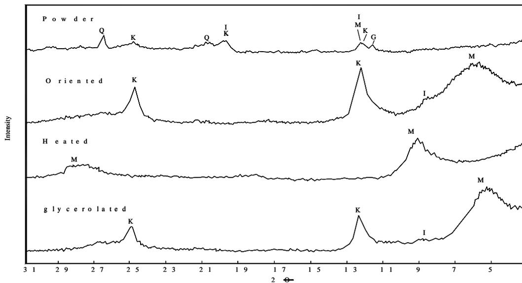
the mineralogical composition of EL- Saff clays agrees with that of the most Egyptian clays. Such clays could be used and workable in several building material industries.
