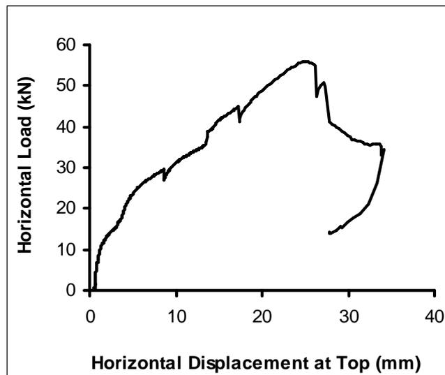
**Fig. 6: Horizontal Load versus Horizontal Displacement for Wall WC**
