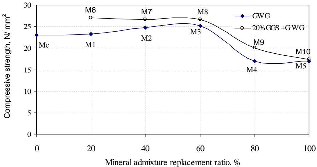
Fig. 1: 7 Day Compressive Strength of the Investigated Mortar Mixtures
