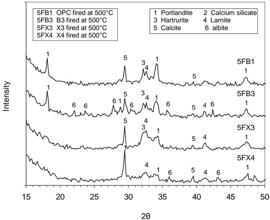
**Fig. 10: XRD Patterns of the Composite -Filled Cement Pastes of OPC, B3, X3 and X4 Fired at 500°C**
