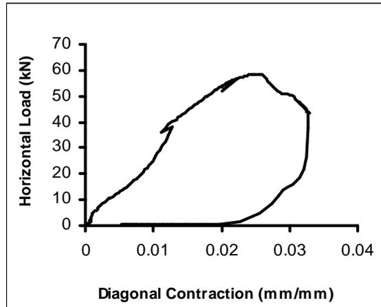
Fig. 10: Horizontal Load versus Diagonal Strain for Wall WG
