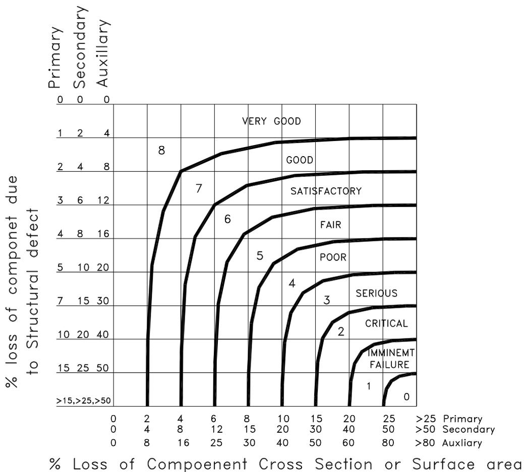
Fig. 4: The Relationship between the Material, Structural Defects and the Proposed Condition Rating.
