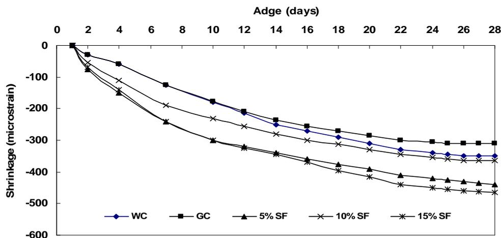
Fig. 5: Free shrinkage behavior of concrete with silica fume
