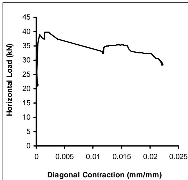
**Fig. 4: Horizontal Load versus Diagonal Strain for Wall WP**
