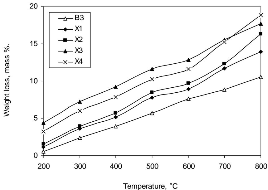
**Fig. 5: Ignition Loss of OPC and Composite - Filled Cement Pastes as a Function of Firing Temperature Up to 800°C**
