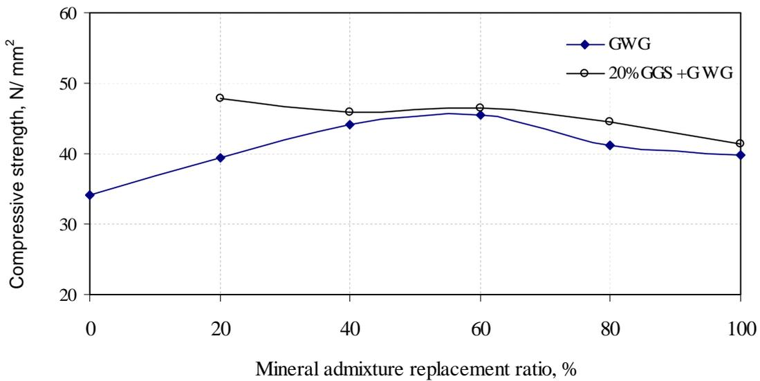
**Fig. 3: 90 Day Compressive Strength of the Investigated Mortar Mixtures**
