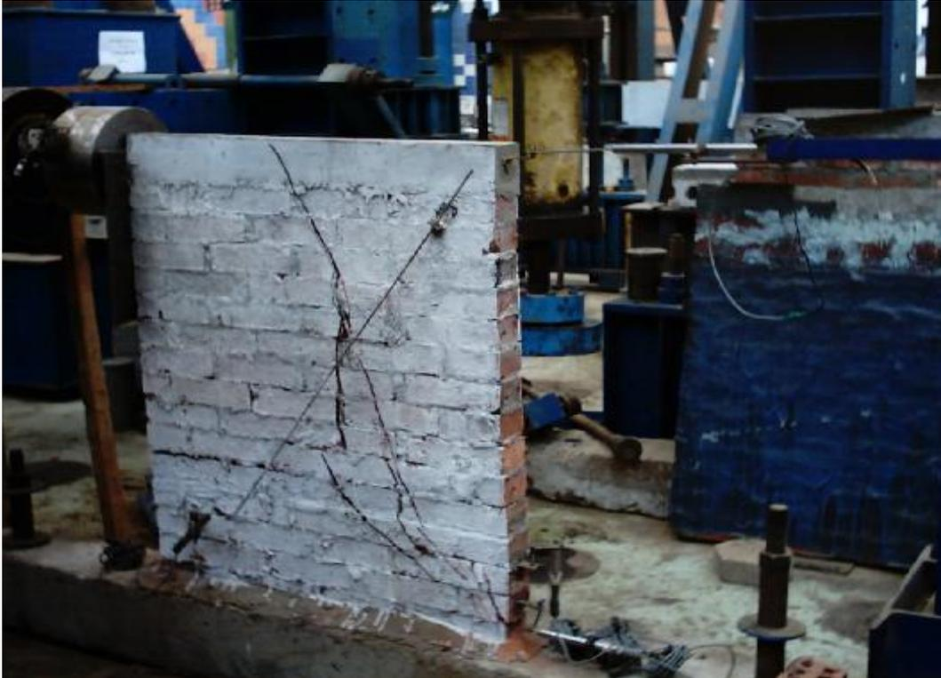
**Fig. 5: Crack Pattern of Wall WP**
