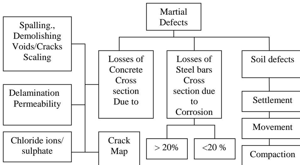
Fig. 2: Material Defects Types in Primary and Secondary/Deck Elements
