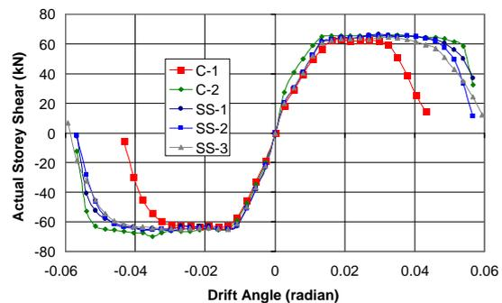
**Fig. 12: Storey Shear Versus Drift Angle**
