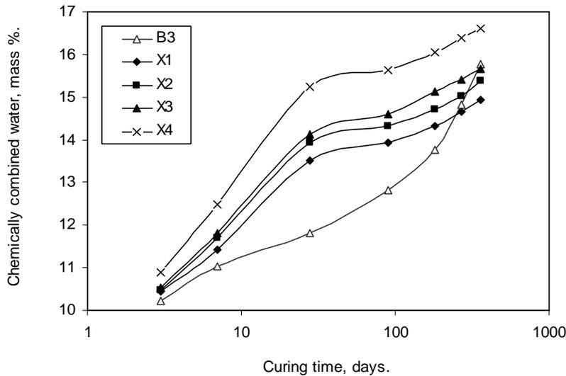
**Fig. 2: Combined Water Content of Composite - Filled Cement Pastes as a Function of Curing Time Up to 360 Days**
