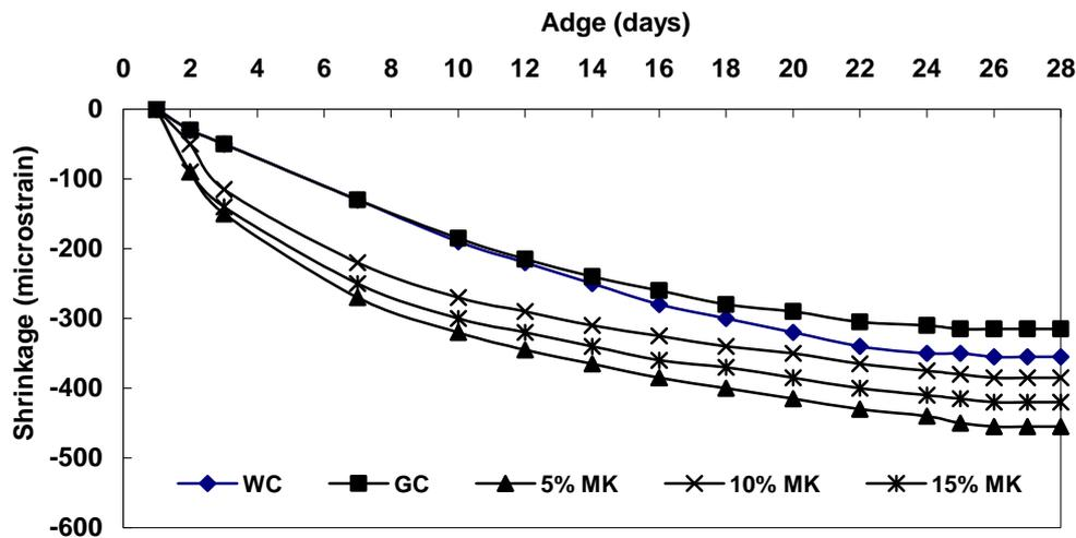
Fig. 6: Free Shrinkage Behavior of Concrete with Metakaolin
