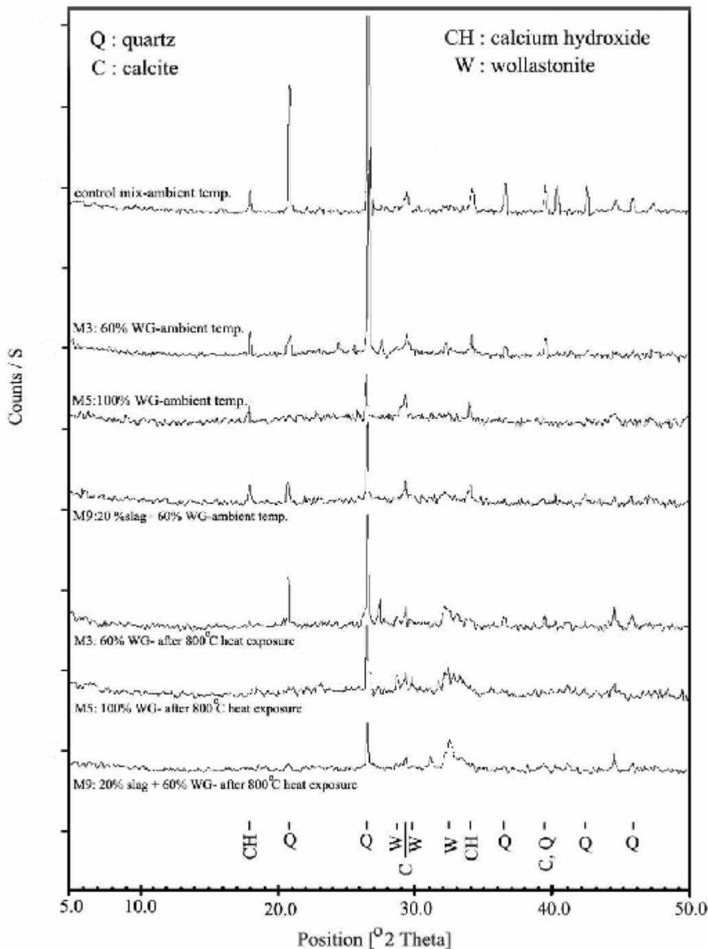
**Fig. 7: X-ray Diffract grams of some of the Investigated Mixes before and after Exposure to Elevated Temperature.**
