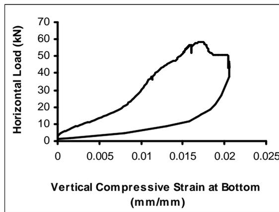
Fig. 11: Horizontal Load versus Vertical Strain at the Heal for Wall WG
