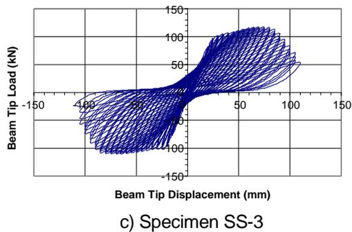
**Fig. 9: Load-Displacement Hysteresis Loops for the Test Specimens**
