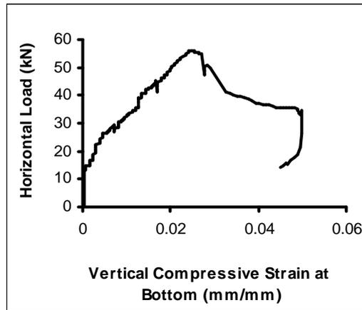
**Fig. 7: Horizontal Load versus Vertical Strain at the Heal for Wall WC**
