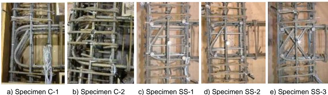
**Fig. 3: Reinforcing Details in Beam-Column Joint Specimens**
