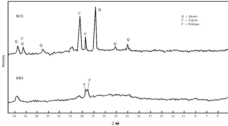
**Fig. 2: X- Ray Diffraction Pattern of the Studied Burnt Rice BRS and Burnt Cotton Straws BCS**
