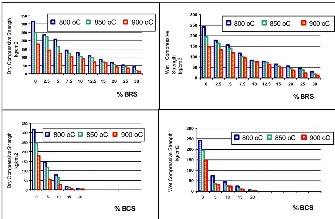
**Fig. 13: Dry and Wet Compressive Strength Values of the Fired Clay Specimens with Different Percentages of Burnt Rice and Cotton Straws BRS and BCS Additives at Different Degrees of Firing.**
