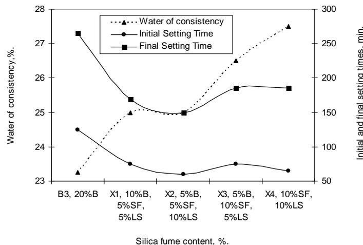
Fig. 1: Water of Consistency, Initial and Final Setting Times of Composite- Filled Cement Pastes as a Function of Mix Composition
