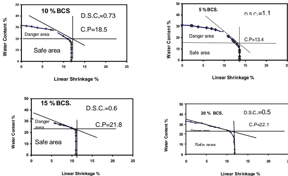
**Fig. 6: Bigot's Curves of the Studied Clay Specimens with Different Percentages of Burnt Cotton Straw BCS additives.**
