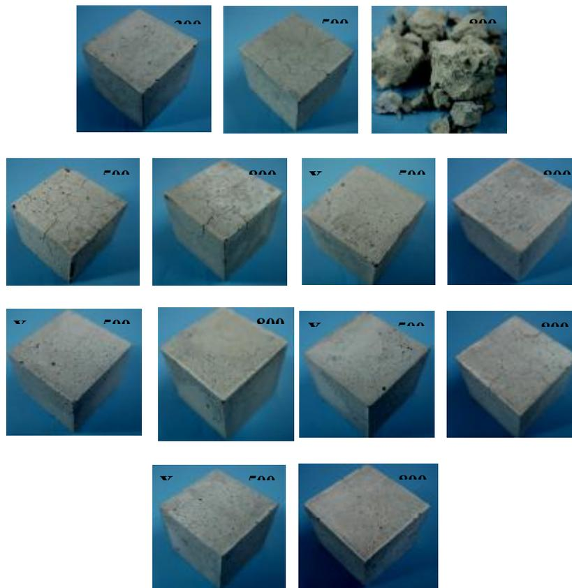
**Fig. 11: Typical Visual Inspection of the Investigated Hardened OPC and Composite - Filled Cement Pastes Fired at 300°, 500° and 800°C**
