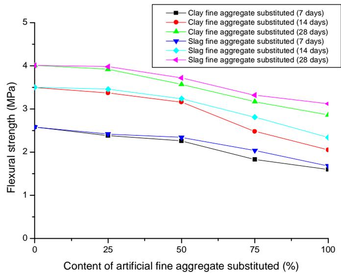
**Fig. 4: Variation of Flexural Strength of Mortars as a Function of the Quantity of Artificial Fine Aggregate Substituted**
