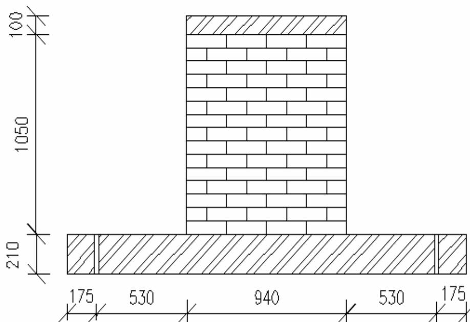
Fig.1: Schematic Drawing of Tested Masonry Walls
