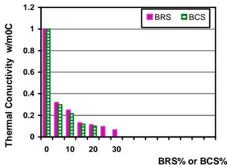
**Fig. 14: Thermal Conductivity of Clay / BRS and clay/BCS Specimens Fired at 850 °C.**
