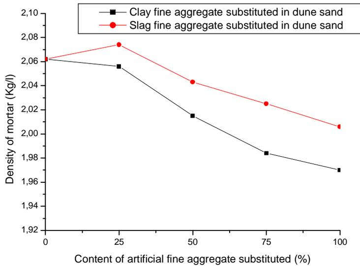
**Fig. 2: Variation of Density as a Function of the Quantity of Artificial Fine Aggregate Substituted**
