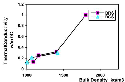
**Fig. 15 Relationship between BRS or BCS Content and Thermal Conductivity of clay/BRS and clay/BCS Specimens Fired at 850 °C.**
