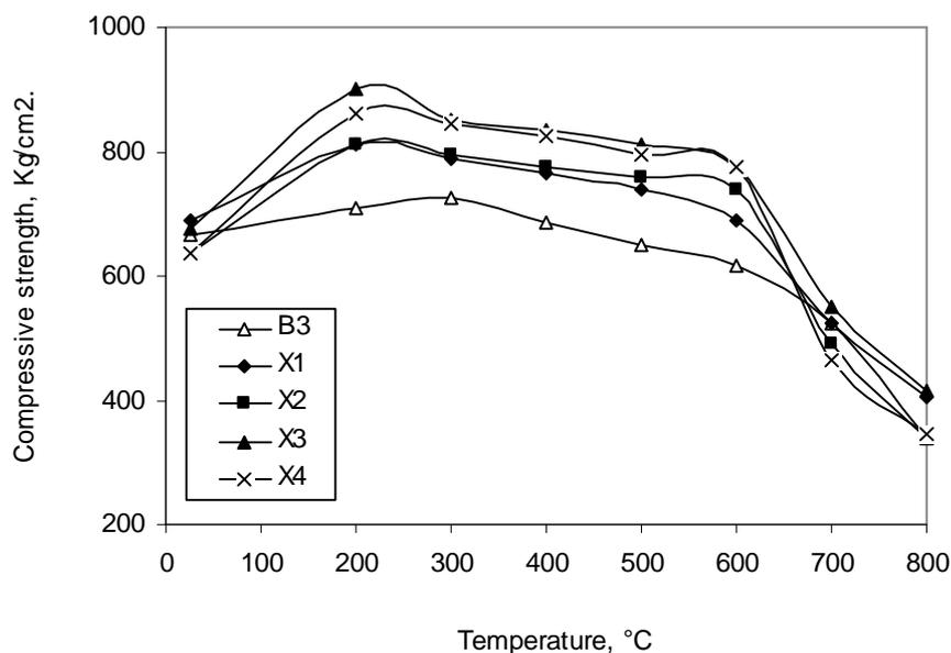
**Fig. 8: Compressive Strength of OPC and Composite -Filled Cement Pastes as a Function of Firing Temperature Up to 800°C**
