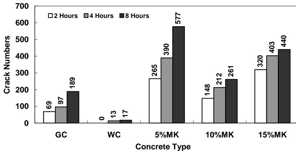
Fig. 3: Number of Cracks with Time for Concrete with Metakaolin.
