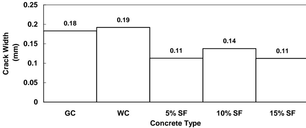
Fig. 2: Average Crack Width at 8 Hours for Concrete with Silica Fume
