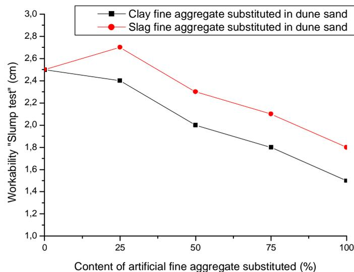
**Fig. 1: Variation of Workability as a Function of the Quantity of Artificial Fine Aggregate Substituted**
