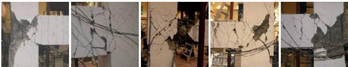
a) Specimen C-1   b) Specimen C-2   c) Specimen SS-1   d) Specimen SS-2   e) Specimen SS-3
