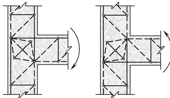
Fig. 4: SST Model with Diagonal Ties in the Joint
